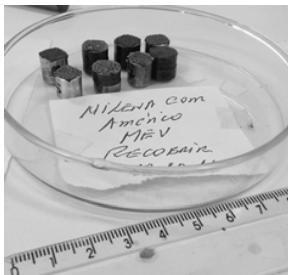
Figure 3 - Soil samples placed on stubs and glued with carbon.
