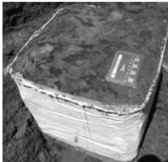
Figure 2 - Undisturbed sample collection using plastics film and plastered bandage.
