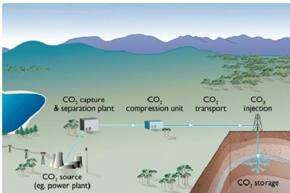
**Illustration 1.** Carbon Capture and Storage Scheme (CleanTechnica, 2011 - <http://cleantechnica.com/>)
